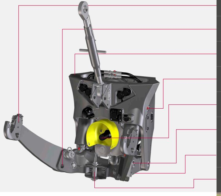
• Electronic Frontlift Control (EFC) is a handy electronic control module for the front linkage and front PTO that allows you to adjust and monitor all front linkage settings from the tractor cab.
